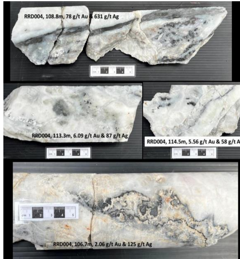
Above: Core photos from interval (106.7-114.5m) of high-grade Au and Ag in RRD004 containing disseminated electrum (TOP) and dark-grey Ag-bearing minerals (CENTER). Segregation of ginguero banded quartz containing abundant disseminated dark-grey sulphides (BOTTOM).
